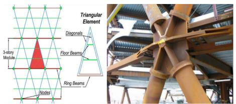
Figure 18. 3-story diagrid module and a triangular element sample(Asadi and Adali,2017) Figure 19. Gherkin Tower node sample(Boake,2016).
