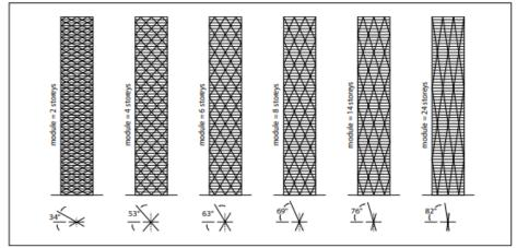
**Figure 20.** Module design with different diagonal lengths and angles that vary depending on the floor-design status of a 60-story building (Boake, 2014).
