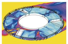
Figure 43. Thermal analysis showing the contribution of the presence of light wells(Sahin Karagöz, 2016).
