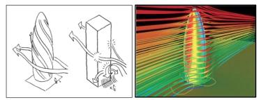
Figure 44. Relation of building form with wind (Boake, 2014).
