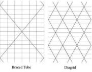
Figure 16.Braced tube vs. Diagrid structure (Moon, Connor, and Fernandez, 2007).
