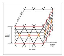
Figure 17. Typical diagrid module(Moon,2011).
